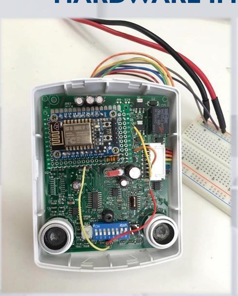
Our final hardware design involves the device integrating directly with an existing occupancy sensor.
